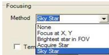
If you select any method other than none, FocusMax will be invoked at the start of every series. A series is a number of exposures corresponding to a specific filter, binning and exposure duration. In addition to that, CCDAutoPilot2 will refocus at whatever time is entered in the Refocus every xx minutes box – automatically. Thus you have complete control over when and how often FocusMax needs to refocus your system. Let’s review each of these Focusing Methods to see which ones to use where.
