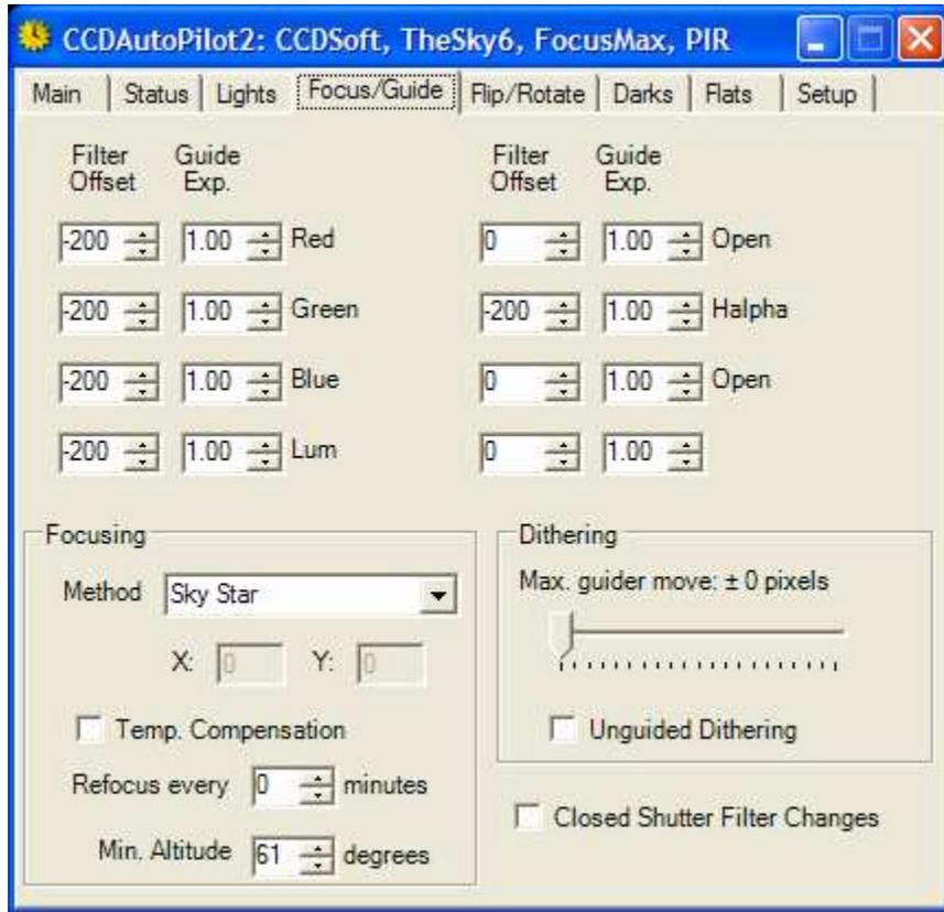
This is the Focus/Guide tab of CCDAutoPilot2. The focuser is controlled via the free program, FocusMax. Options exist for the open loop techniques such as filter offsets and temperature compensation. CCDAutoPilot2 adds a number of closed-loop focusing options shown here:
